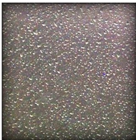
Figure 1.2 On the untreated metal sheet, the water simply remains, as clearly indicated by the many water drops. This leads to the formation of rust.
